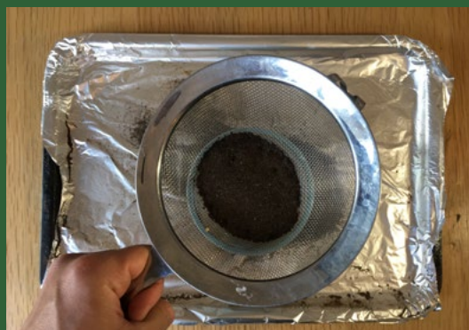
2. Sieve the dried mud in a fine sieve two or three times to discard the larger granules.
