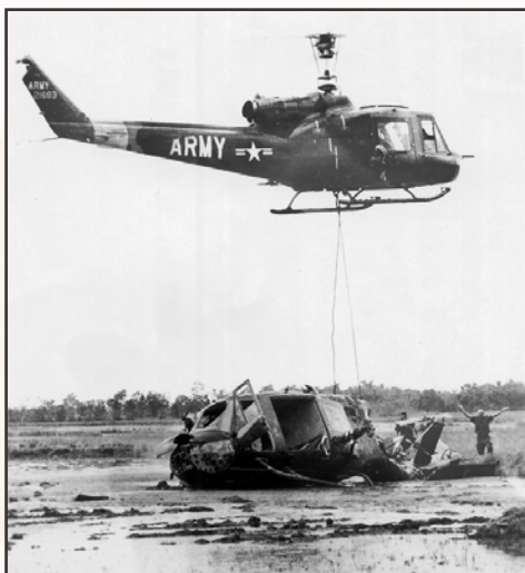
Above: Salvage operation: a US Army UH-1 Iroquois helicopter retrieves another, downed during the battle of Ap Bac, January 1963.
