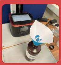
1. My previous print finished with plenty of resin left in the tank, but it also failed to print in one area. I could run another print with this resin but suspect parts could be hiding under the surface, so I prepare my funnel and filter.
