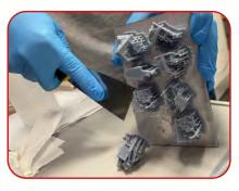
3. The prints can be removed from the build plate with a little gentle encouragement! Notice I'm working over a flexible mat which will help me with workstation clean up later.
