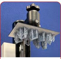
1. With the print complete the build plate is ready to be unscrewed from the printer.
