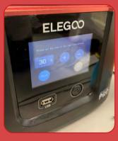
2. The tank clean function should only need to run for 30 seconds.
