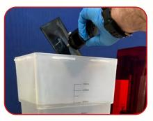
If you are using all ELEGOO kit their cleaning station is designed to hold the build plate and whatever is on it. This can make the cleaning process a lot easier and saves you needing to remove the prints until after they are cleaned.
