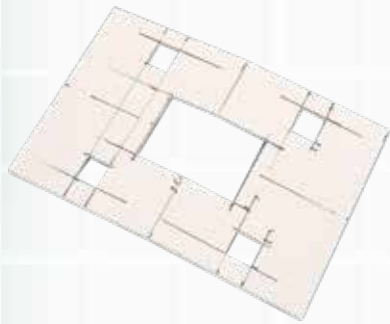
6) The roof for the upper building followed a similar technique, with four apertures to take the uprights of frame B, and a large central aperture through which frame C fits.
