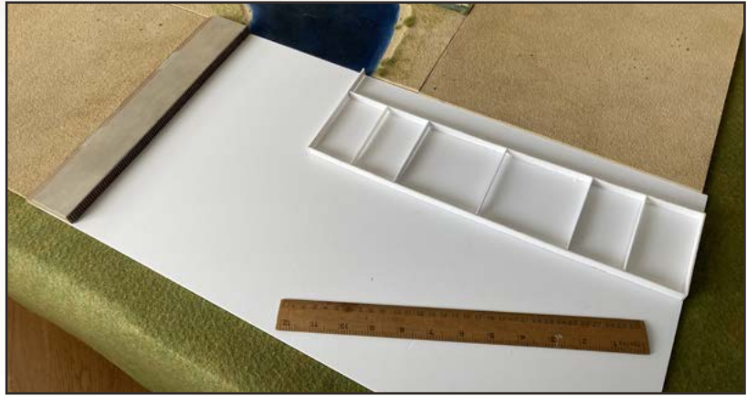
Above: Plasticard provided the skeleton for the quay and promenade area of the dock.
