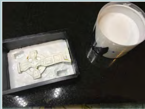
4) Making a mould of the finished cross for replication.
