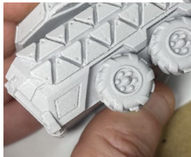
Left: Some stepping shows on the wheels and vehicle side, though it will be greatly softened with primer and paint.
