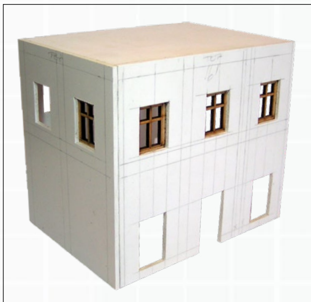
3. I used the Sarissa laser-cut MDF windows and glued them in place behind the main window openings. I used superglue to hold the window frames in place and made sure that the frames were square in the openings. Superglue was also used to glue the walls together.
