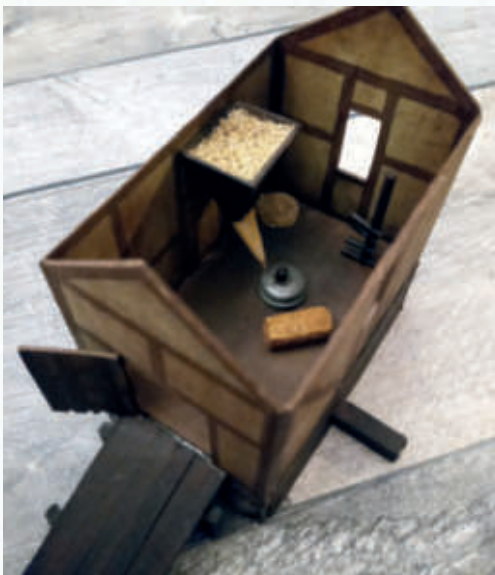
Above: Internal view with the hopper in place.
