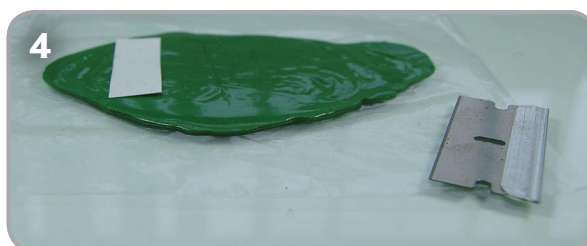
4. When nearly dry, remove top layer of plastic sheet. I have used a paper template as a basic former and cut out the required shape with a razor blade.
