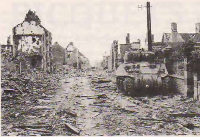
(3) A knocked out Sharpshooters' Sherman, the shell entered on the left side of the turret. Also note the 7th Armoured Division 'Desert Rat' shield on the left and the Browning machine gun lying in the road. The two Tigers are just visible in the distance. (Imperial War Museum)
